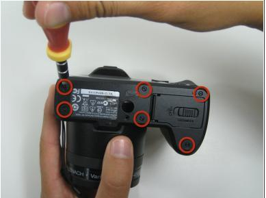
After removing the screws located on the right side, remove the six screws located on the bottom
