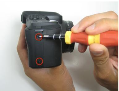
Next, remove the two screws located on the right side of the camera.
