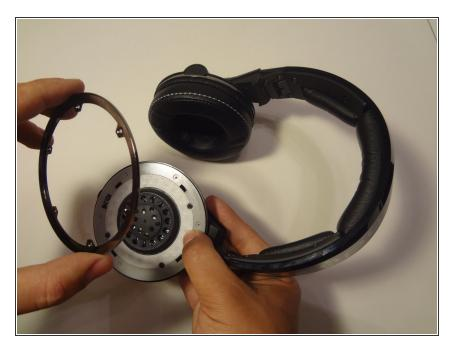
Using your screw driver, remove the six Philips 2mm screws located on the chrome ring.
