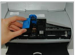
• Grab the ink cartridge and remove it from the printer.
