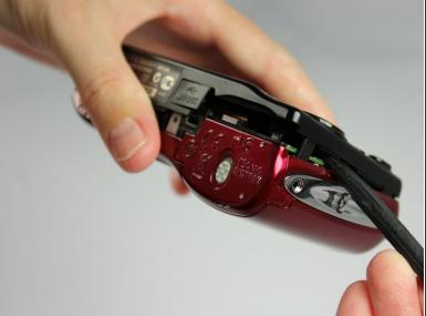
Wedge the flat end of the spudger in between the front and back cover. Carefully push the spudger downward, which will lift the back cover off the camera.
