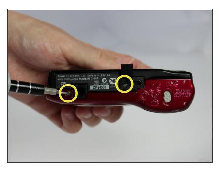
Flip over the rubber AV cover at the bottom of the camera. Unscrew the last two 2mm screws on the bottom of the camera.
