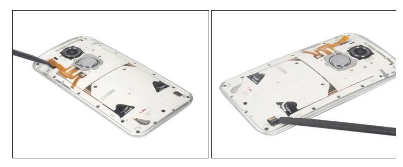
• Release the power button connecting flex connector and battery connector carefully.
