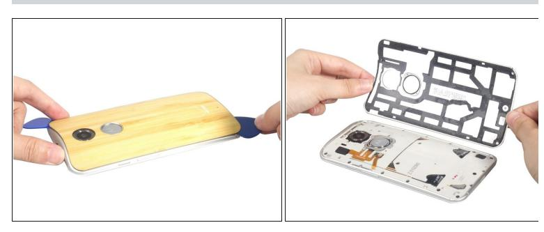
Slide the guitar pick to cut the adhesive sticker and peel off the back cover.
