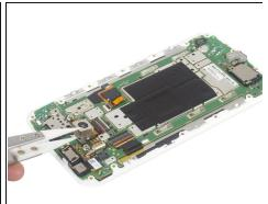
Release rear camera connector and remove it easily.
