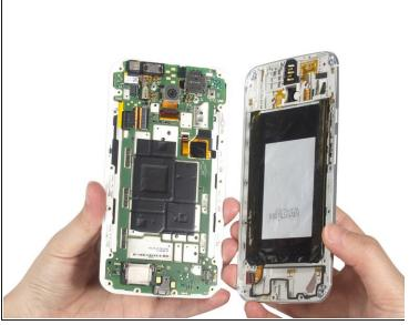
Twist off all 18 black torx screws and separate the middle housing from front assembly.
