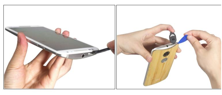
• Push the eject pin to open a gap and place a guitar pick into the gap.
