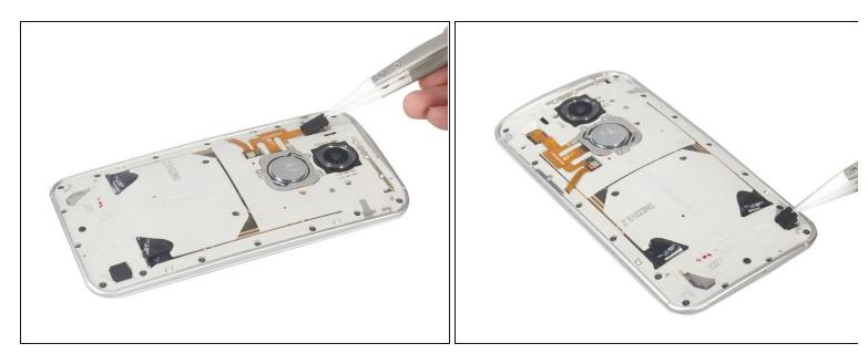
• Remove two pieces rubber cover which protecting the flex connectors.
