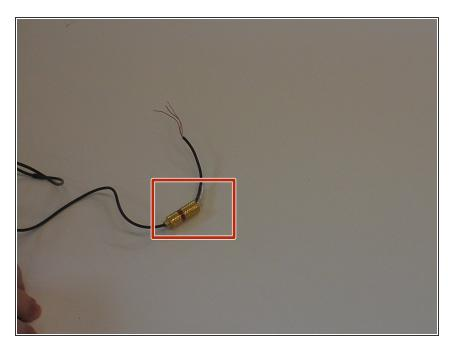
Put the exposed cord through the metal and plastic sleeves of the jack, as shown.
