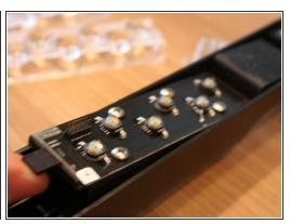
Now you can CAREFULLY take out the LED assembly. It's attached to a metal heat dissapating bracket. CAREFUL with the wiring. Note that the bracket is retained by the plastic housing. It might need some help before it gives way.
