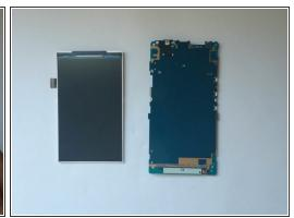
Release the LCD display from the main board.
