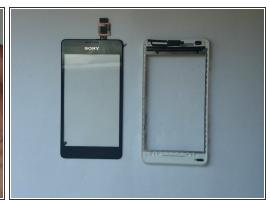
Use a plastic tool for separating the glass from the frame.
