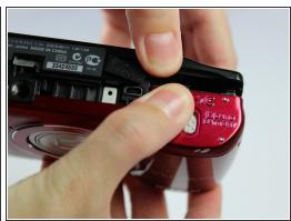
Using your hands, open the camera slightly by using the indentation above the camera compartment.
