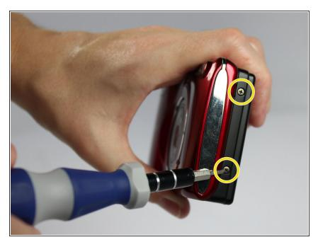
Unscrew the two 2mm screws on the opposite side.
