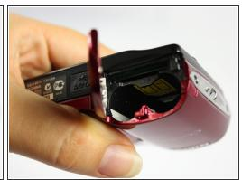
Remove the batteries from the battery compartment by sliding the white battery compartment switch up and then move the panel toward the right.
