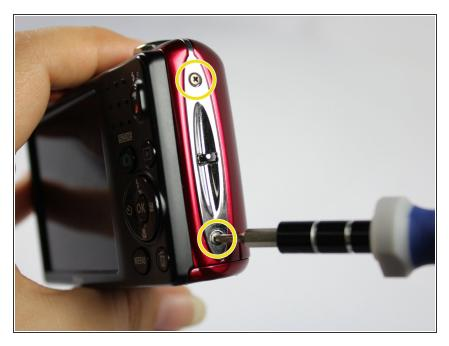
Using the Phillips #000 screwdriver, unscrew the two 2mm screws next to the battery compartment on the right side of the camera.
