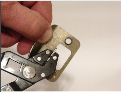
Take the strike plate and put it in your hand. Using the pliers in your other hand, bend the metal tab toward the flat side of the strike plate.
