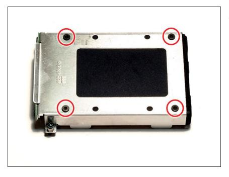
Remove the four T8 Torx screws from the hard drive bracket.
