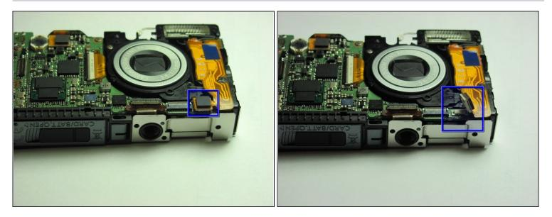
• Disconnect the connector at the bottom of the camera that attaches the flash to the motherboard by gripping it with you fingers and flipping it up.
