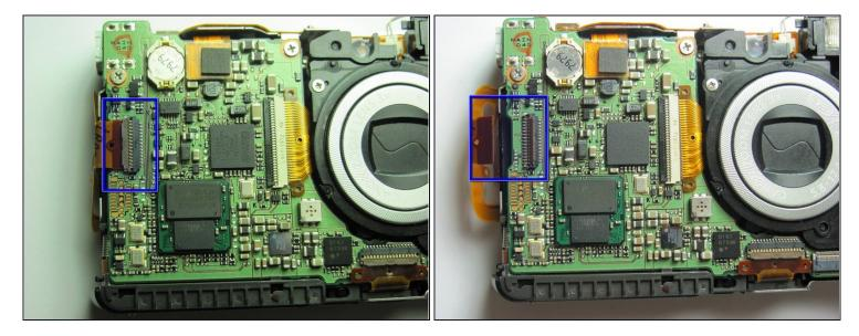
• Disconnect the ribbon that attaches to the left side of the motherboard by flipping up the ZIF connector and then sliding the ribbon out.
