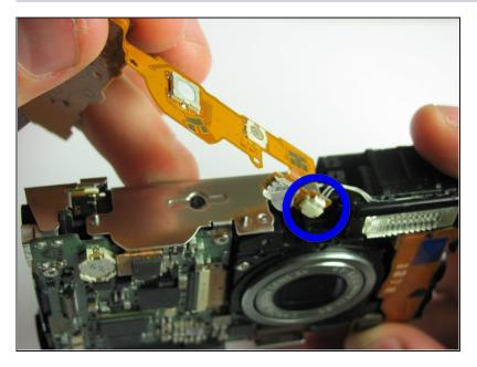
• Disconnect the white connector on the top right side of the camera by pulling the wire out of the connector with your fingers.
