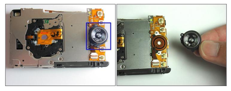
• Remove the plastic and rubber circular button from the back of the camera by lifting it with your fingers.
