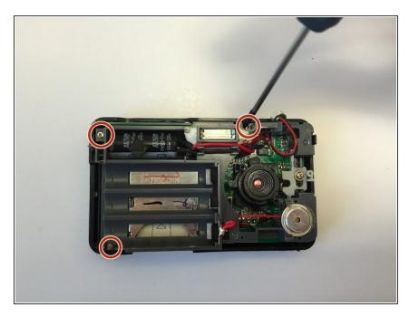
Remove the three 2 mm screws holding in the gray plastic cover, using a Phillips #00 screwdriver.
