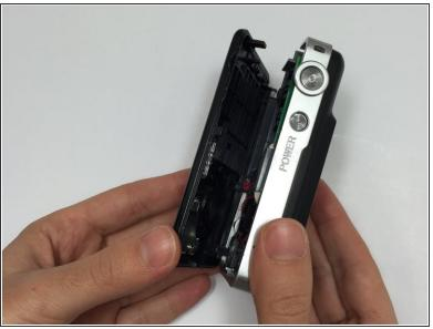
Separate the front piece of the camera from the back to reveal the motherboard.
