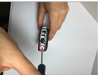
Remove the 3 mm screws on the sides of the camera, using a Phillips #00 screwdriver.
