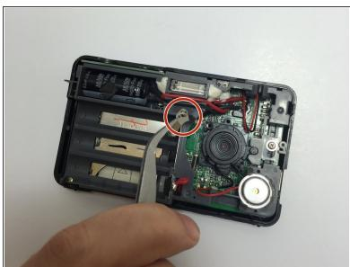
Remove the two silver plates using tweezers.
