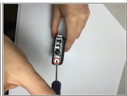
Use a Phillips #00 screwdriver to remove the 3 mm screws at the sides of the camera.
