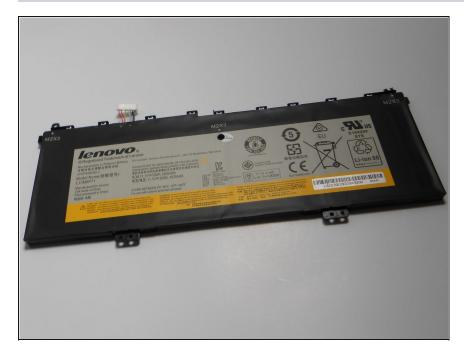
• Once all wires are unattached to the rest of the computer, remove the battery from the laptop and replace.
