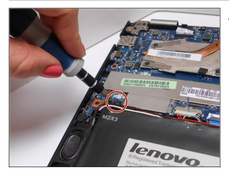
• To remove the battery, use a Phillips head screwdriver to unscrew three 3.175 mm screws. One will be in the center of the battery (covered by a Lenovo sticker) and the other two are in the corners.
