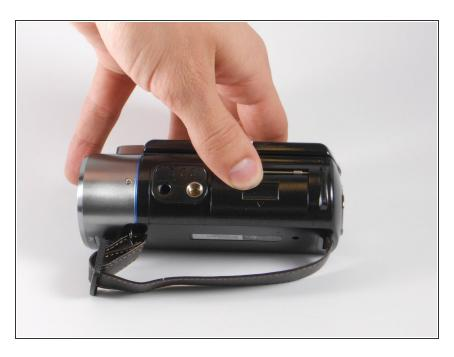
Locate the arrow marked on the battery slot door and push in the direction the arrow points to open the latch.
