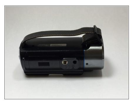
Locate the battery slot on the underside of the camcorder.
