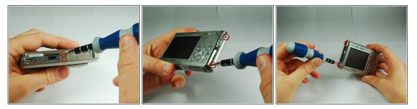
(i) There are two screws on the left and right sides of the camera, and two screws on the bottom.
