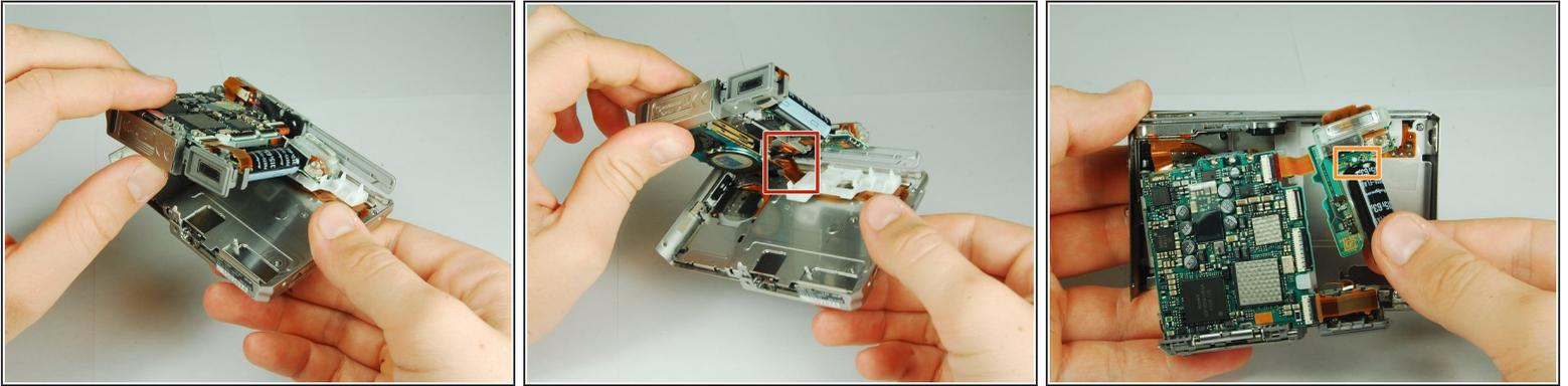
**⚠** This camera houses a very strong capacitor (the black cylinder). Avoid touching anything around the two wires coming out of the top. Doing so will risk serious electric shock.
