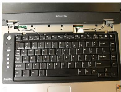
Remove the top panel by popping the panel out the top left socket, then do the same with the right side.
