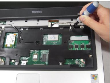
Remove the 3.76mm screw from the ground wire.
