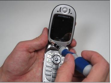
Remove the four 3.8 mm T-6 Torx screws.
