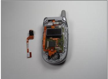
• Lift the top ribbon cable, with camera attached, up and away from the rest of the phone.
