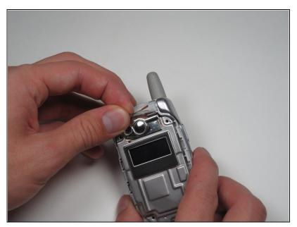
Gently peel off the plastic film from the metal plate above the camera lens as shown.
