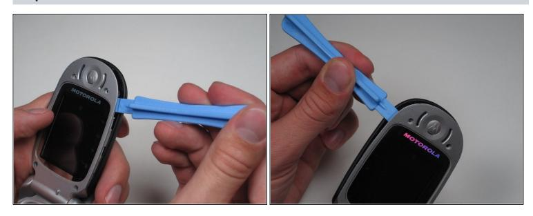
Separate the cover from the edges using a plastic opening tool.
