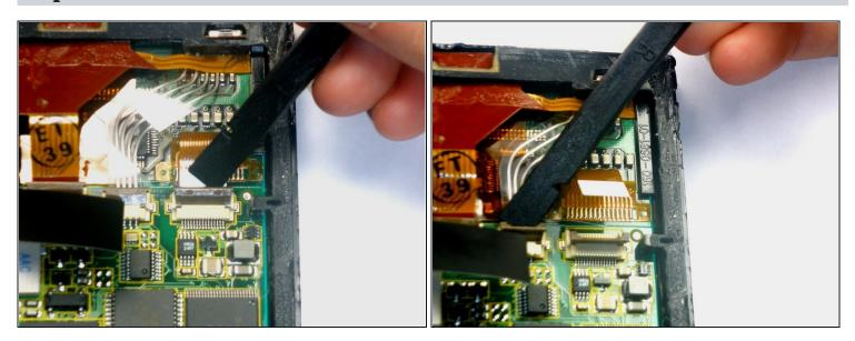
• Using the spudger lift the tabs holding the LCD/Digitizer combo cables to the WorkPad.
