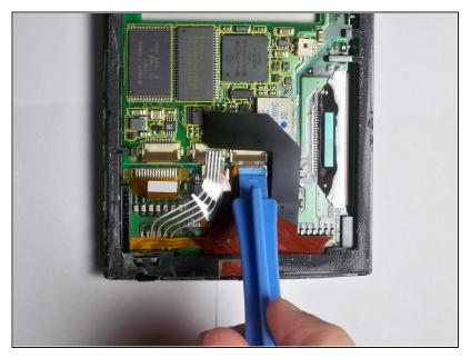
Using the plastic opening tool, lift the clip holding the motherboard cable.
