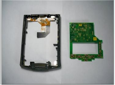
• Gripping the motherboard as shown, lift up slightly and pull outward.
