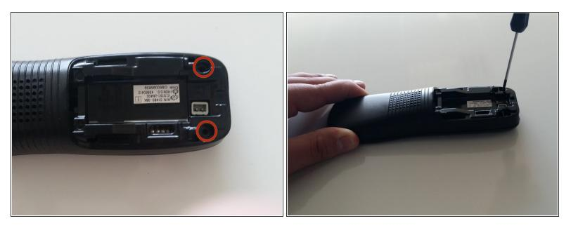
• Remove the two 9mm Phillips #1 screws in the battery compartment.
