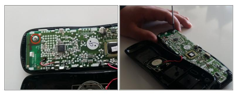
• Carefully remove the 9mm Phillips #1 screw from the top corner of the circuit board.
