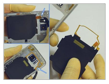
Pry up the charging chip flex ribbons on both sides of rear housing. (Notice: be careful not to damage the flex ribbons.)
