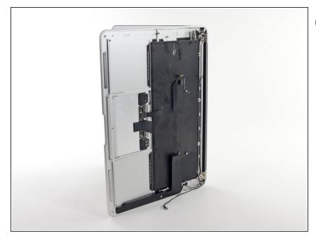
(i) Open the display so that it is perpendicular to the upper case and place it on a table as shown.
