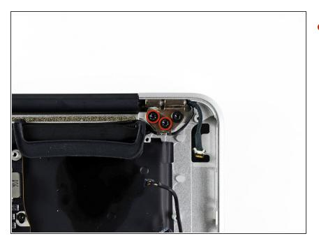
Remove the inner two 4.9 mm T8 Torx screws securing the antenna cable retainer and left clutch hinge to the upper case.
