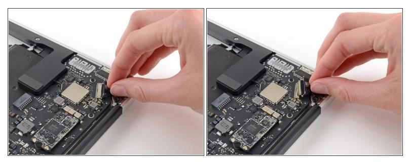
• Pull the display data cable connector straight away from its socket.
