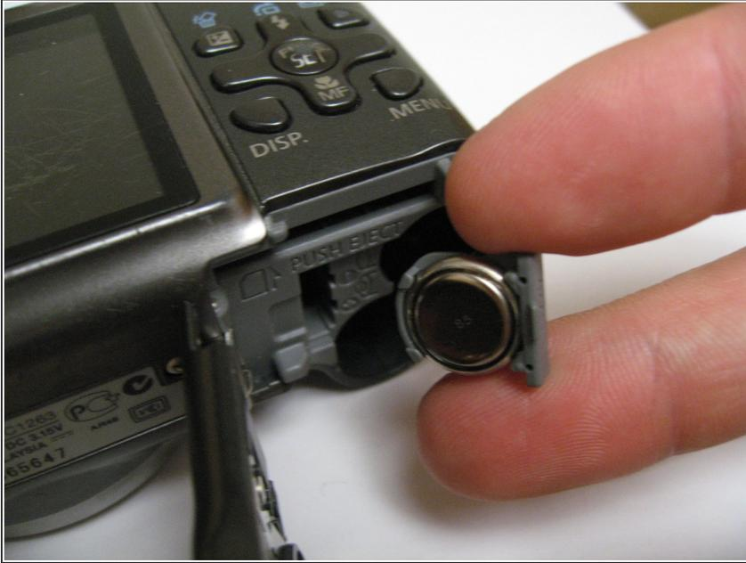
**⚠** When replacing the clock battery, be sure to have the battery oriented properly, as shown in the picture.
