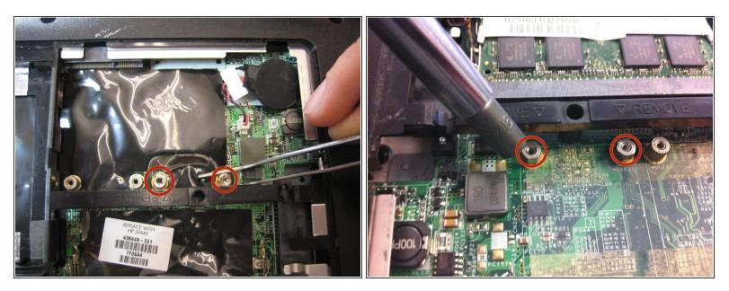
Use a pair of tweezers (or 3/16 nut driver) to remove the two 5mm hex screws secured to the logic board.
