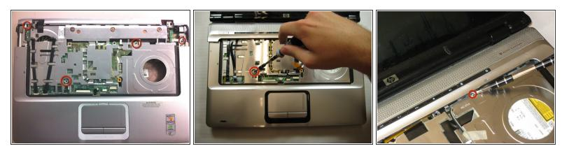
Remove the four 5.8 mm Phillips screws securing the top cover to the lower case.
