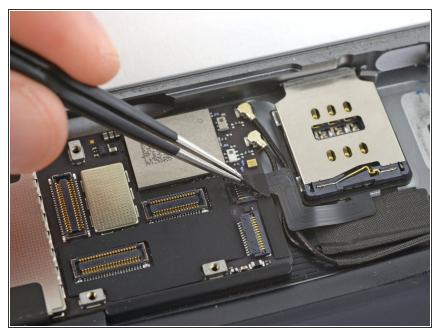
Use tweezers to peel and remove the piece of tape covering the SIM board cable connector on the logic board.
