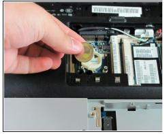
• Remove the RTC Battery from the battery holder.
