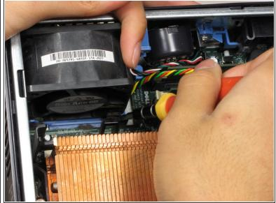
Remove the rubber grommets from the base of the fan. A screwdriver or spudger may be useful.
