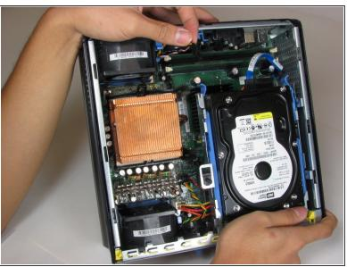
Remove the power supply that connects the upper fan to the motherboard. The power supply has black, red, green and yellow wires.
