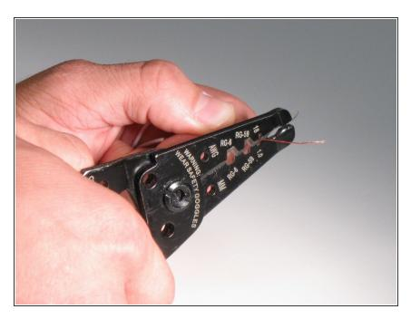
• Remove the enamel from the red and blue wires with a wire stripper.
