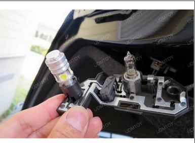
Remove the bulb and swap it out with the new LED bulb.
