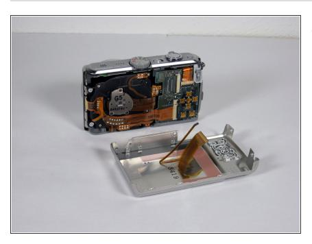
Remove the back casing from the camera.
