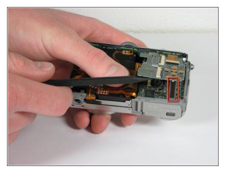
Carefully unsnap the front logic board from the rear logic board using a spudger.
