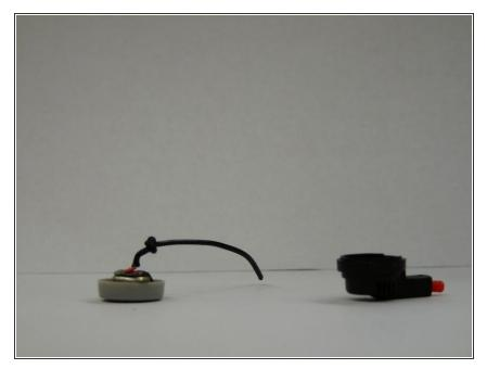
Gently remove the driver unit and wire from the (Black) receptacle part with small pliers or suitable small hand tool.
