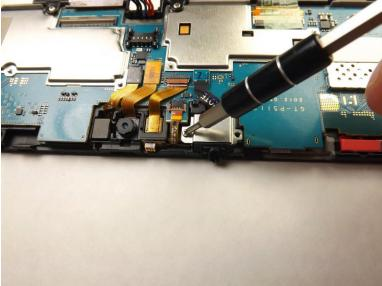
Unscrew the two 3mm screws with the Phillips 000 screwdriver.
