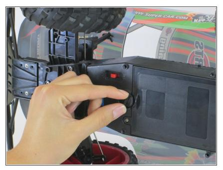
Beginning at the bottom of the truck, twist the release clip on the casing until the release clip is no longer covering the battery casing.
