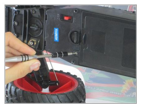
Next, use a Phillips 00 screwdriver to remove the 8mm screw on the battery casing and remove the battery casing.
