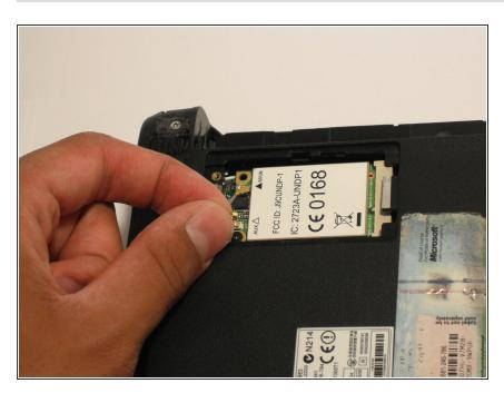
Disconnect the two antenna cables from the left side of the wireless card.
