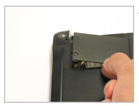
Lift up the panel and remove it from the case.
