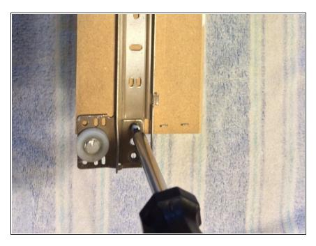
Re-attach the wheel tracks with a screwdriver and screws.
