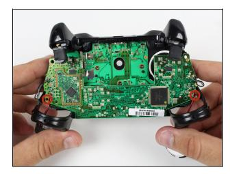
Unscrew the two 7mm T6 screws located near the rumble motor sockets.
