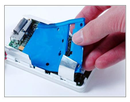
Lift the blue hard drive mounting bracket out of the iPod.
