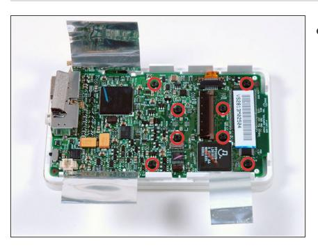
Reove the 8 T6 Torx screws from the logic board.
