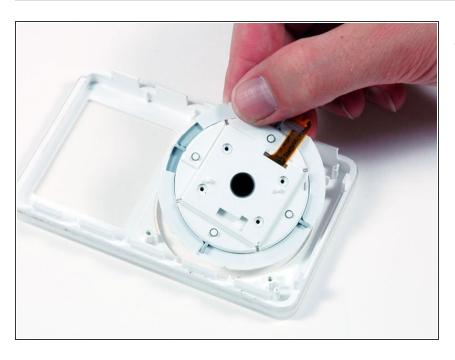
Lift the touch wheel out of the front panel
