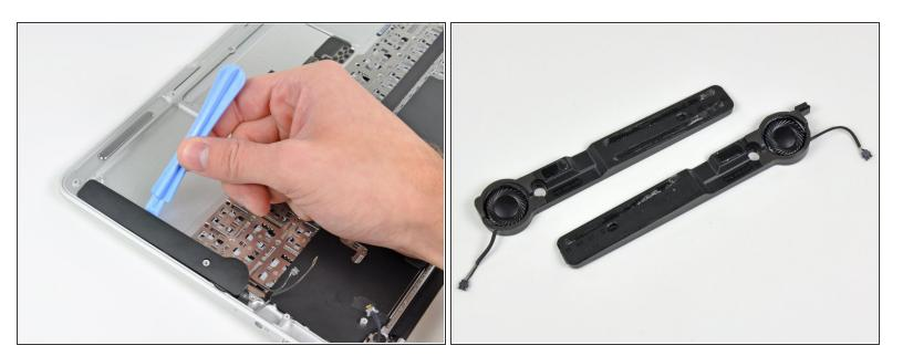
With the help of a plastic opening tool, the speakers come out next. These stereo units pump out...
