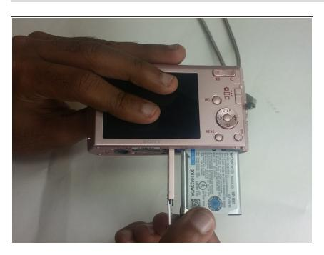
Pull out the battery and replace the new battery.
