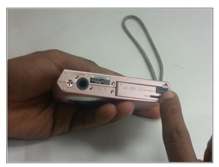
Locate the battery gate and push the button to "open"
