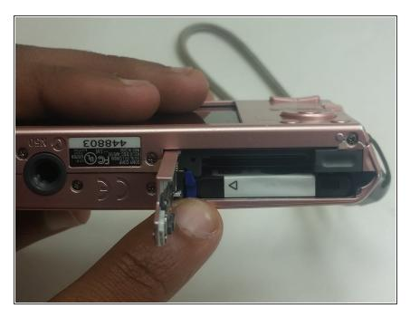
Locate and pull the blue lever back to eject the battery.
