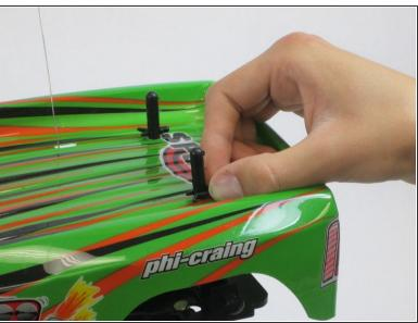
From the top view, remove each of the four pins that hold the casing in place.
