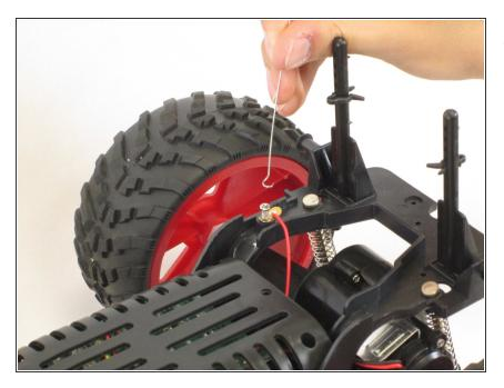
Carefully slide the antenna out from under the screw and remove.
