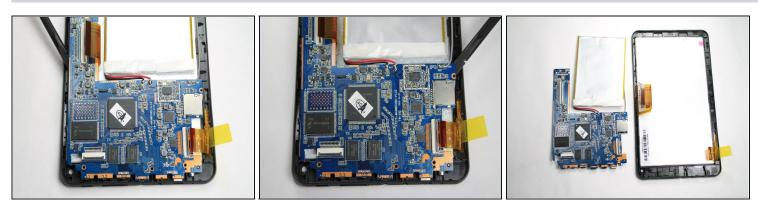
• Gently slide the spudger below the logic board at the left side nearest the battery. Lift upward and away from the power button and bottom connectors.
