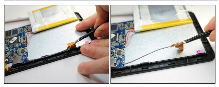
• Gently peel the WIFI Antenna up using a pair of <u>tweezers</u>.
