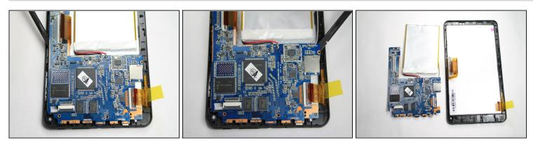
• Gently slide the spudger below the logic board at the left side nearest the battery. Lift upward and away from the power button and bottom connectors.
