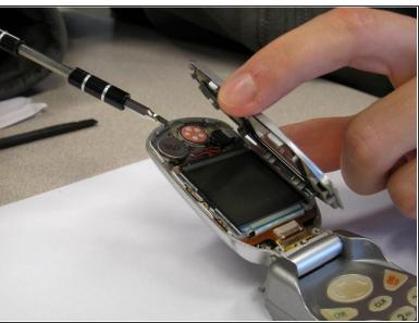
Pry off the screen front cover with a small flathead screwdriver.
