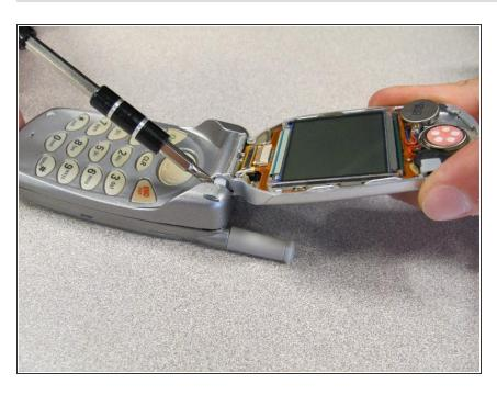
Insert a small flathead screwdriver into the hinge and separate hinge connection.
