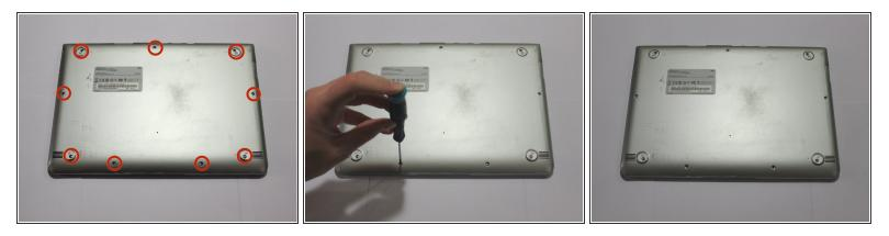
• Remove the nine 4.7 mm screws on the bottom cover using a Phillips #00 screwdriver.
