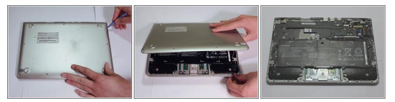
• Pry off the bottom cover using a plastic opening tool.
