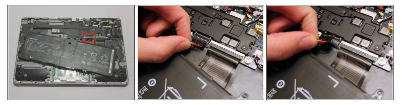
• Disconnect the battery connector by pulling straight up at its base.
