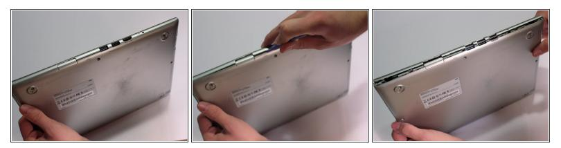
• Pry up the plastic strip on the back of the Chromebook using a plastic opening tool.
