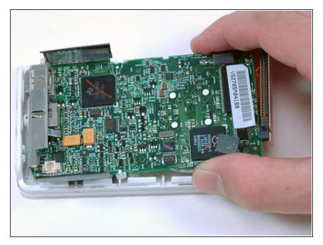
Slide the logic board away from the port end of the casing and lift it out of the iPod.
