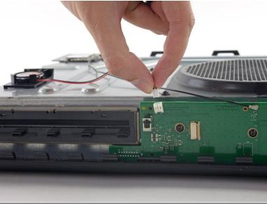
Gently pull up on the speaker cable connector to disconnect it from the front panel board.
