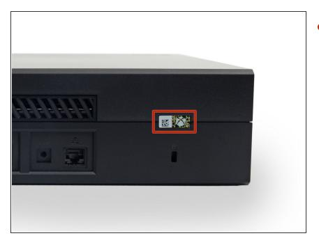
To open your Xbox, you're going to have to cut or peel up this tamper-evident tape. But don't worry
