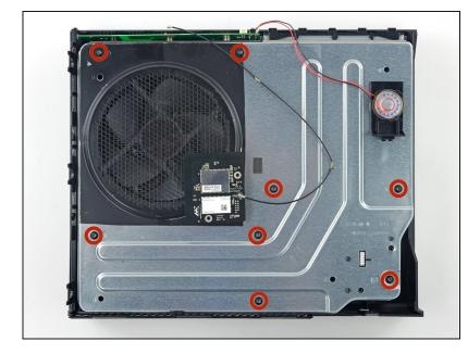
Remove the eight 65 mm Torx T10 screws from the top of the upper metal case.
