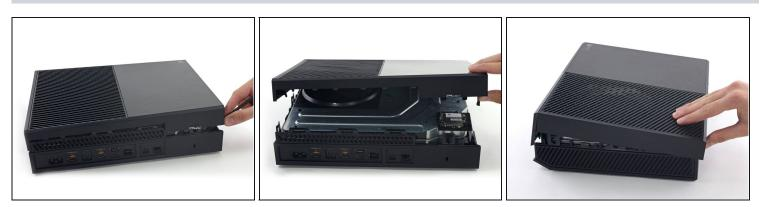
• Starting with the spudger you left in the crack, pry the upper case up to free the last few clips.
