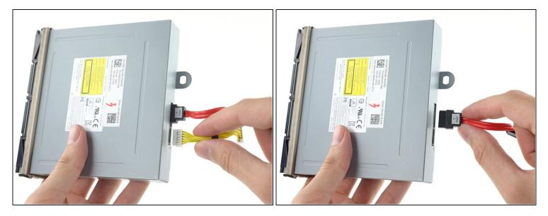
• Remove the optical drive power and SATA data cables.
