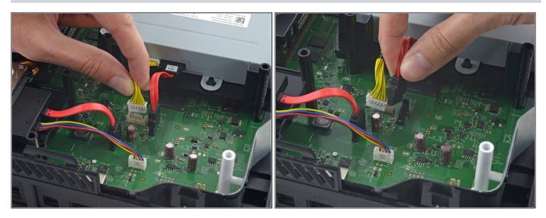
• Disconnect the optical drive power and SATA data cables from the motherboard.
