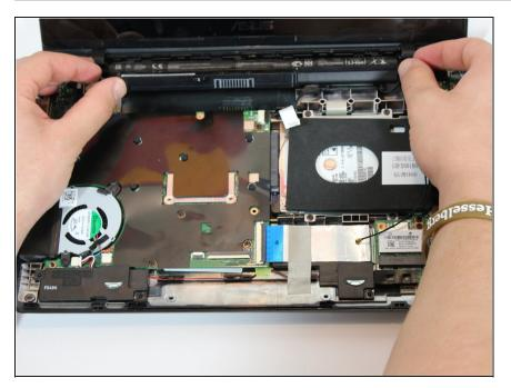
• Slide the battery up and out.
